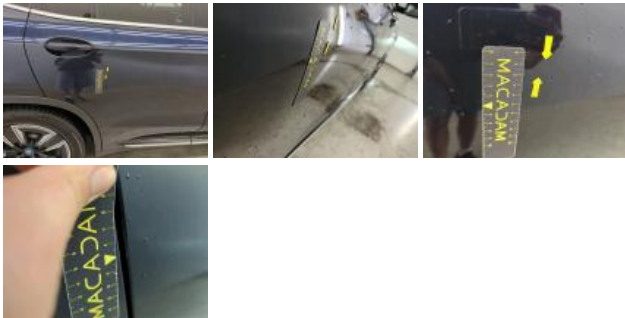
Outer door handle RR, Scratch(es), Repair and paint (complete)
