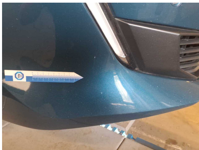
Damage 8: Front bumper: Front bumper - Scratched - Paint
