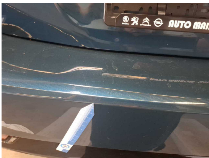
Damage 4: Rear bumper: Rear bumper (Lacknebel+kratzer) - Scratched - Smart repair
