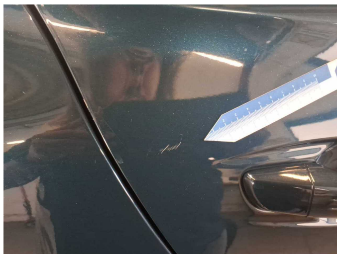
Damage 9: Door - rear right side: Door - Scratched - Paint
