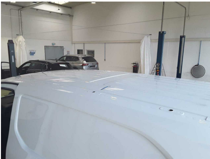
Damage 3: Roof: Roof - dent(s) - Smart repair
