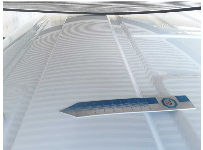
Damage 3: Roof: Roof - dent(s) - Smart repair
