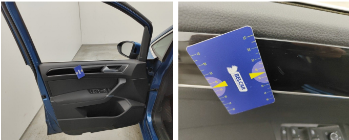
Front Left Door Interior Coating // Replace Completely-scratch
