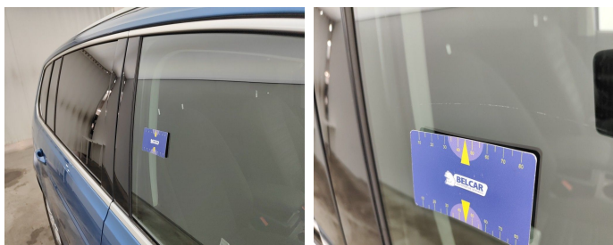
Door Front Right / Window / Replace-scratch
