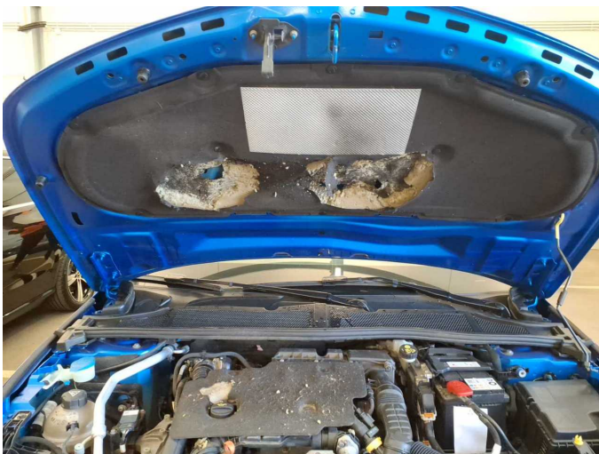
Damage 3: Bonnet: Insulation lining - Broken / torn - Replace
