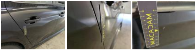
Door FR, Scratch(es), Repair and paint (complete)
