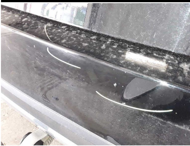
Damage #8: Rear bumper: Rear bumper - Scratched - Repair and paint
