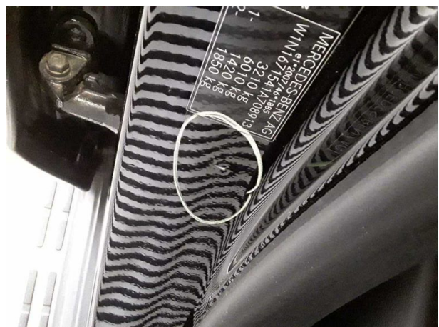
Damage #5: Sill - right side: Sill - Dent / paintcoat damage - Smart repair
