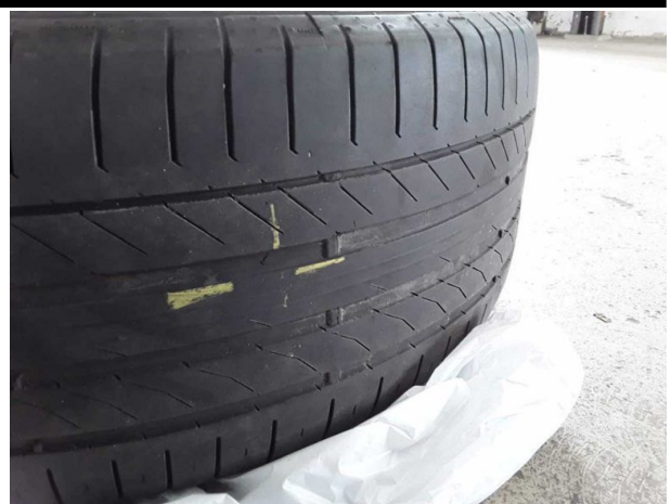
Damage #6: 2nd wheel set: 2 tyres - Worn - Replace
