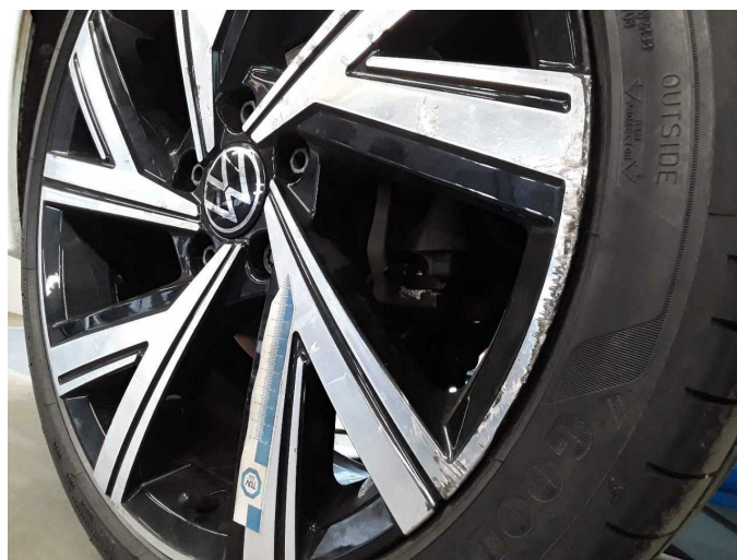
Damage 18: Wheel / tyres: Wheel rims - complete set - Scratched - Replace
