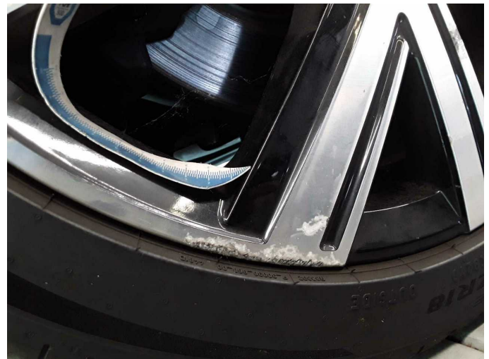
Damage 18: Wheel / tyres: Wheel rims - complete set - Scratched - Replace
