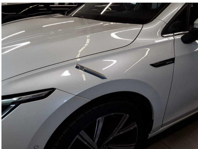
Damage 17: Mudguard - left side: Mudguard - left side - Dent / paintcoat damage - Repair and paint
