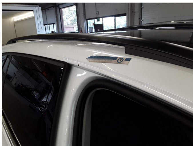
Damage 9: Roof: Roof rail - right side - Corrosion - Smart repair
