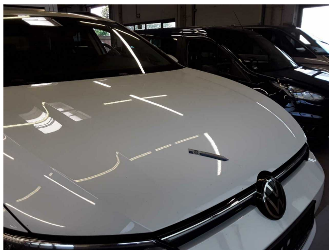
Damage 16: Bonnet: Bonnet - Dent / paintcoat damage - Repair and paint
