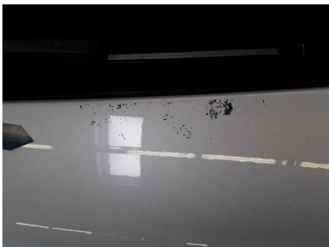
Damage 8: Boot lid / rear door: Boot lid - Paint defect - Smart repair
