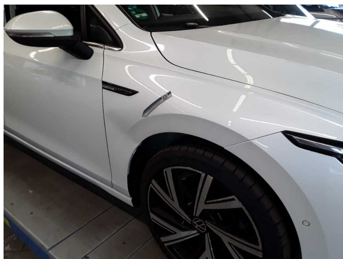
Damage 15: Mudguard - right side: Mudguard - right side - Deformed - Replace
