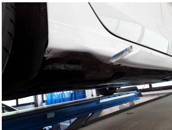
Damage 13: Sill - right side: Sill - Deformed - Repair and paint
