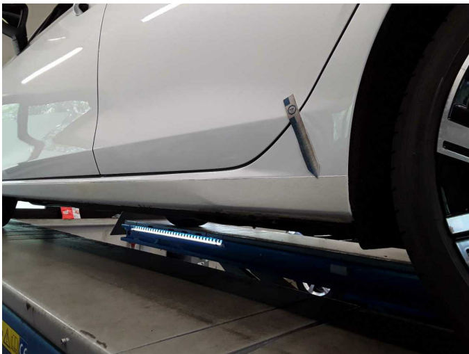
Damage 12: Sill - left side: Sill (Farbabweichung) - Unprofessionally repaired - Paint
