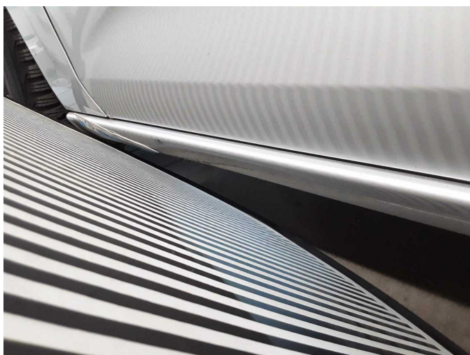
Damage 7: Sill - left side: Sill - Damaged - Repair and paint
