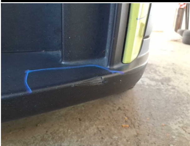
Damage #4: Front bumper: Spoiler - Scratched - Replace
