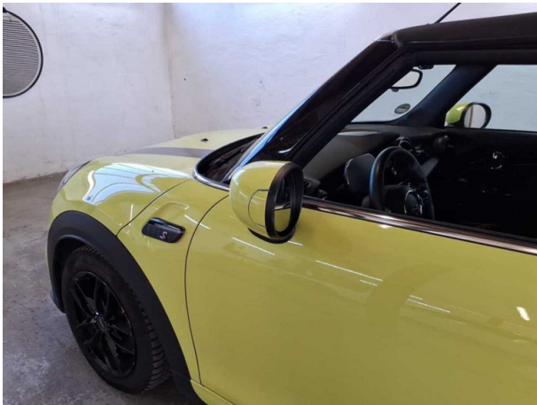
Damage #6: Wing mirror - left side: Mirror housing - Damaged - Replace
