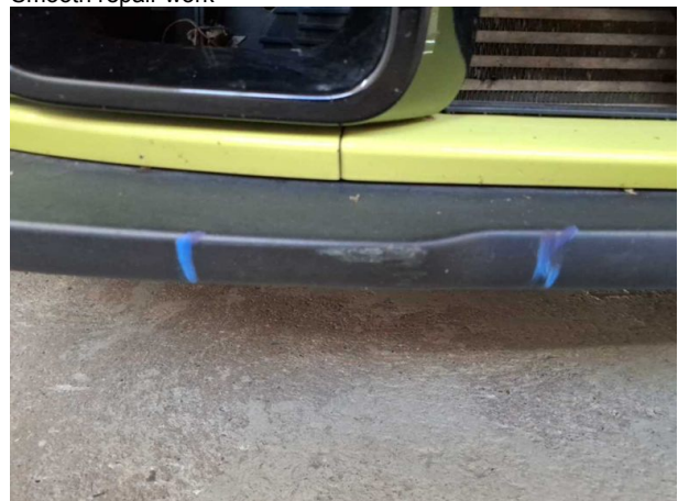
Damage #4: Front bumper: Spoiler - Scratched - Replace
