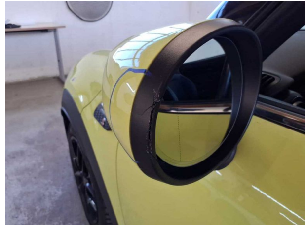
Damage #6: Wing mirror - left side: Mirror housing - Damage... Replace
