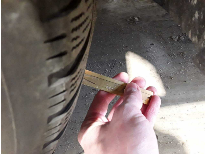
Wear and tear 4: Wheel / tyres: Tyre - front (Kein Teil der Ausstattung) - Does not meet the leasing specifications - No deduction
