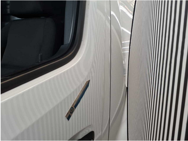
Beschädigung #5: Tür vorn links: Tür - Delle(n) - Smart Repair
