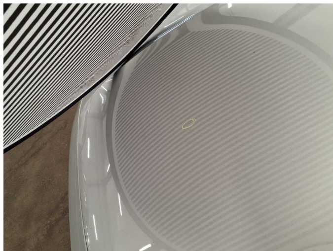
Damage 1: Bonnet: Bonnet - dent(s) - No deduction
