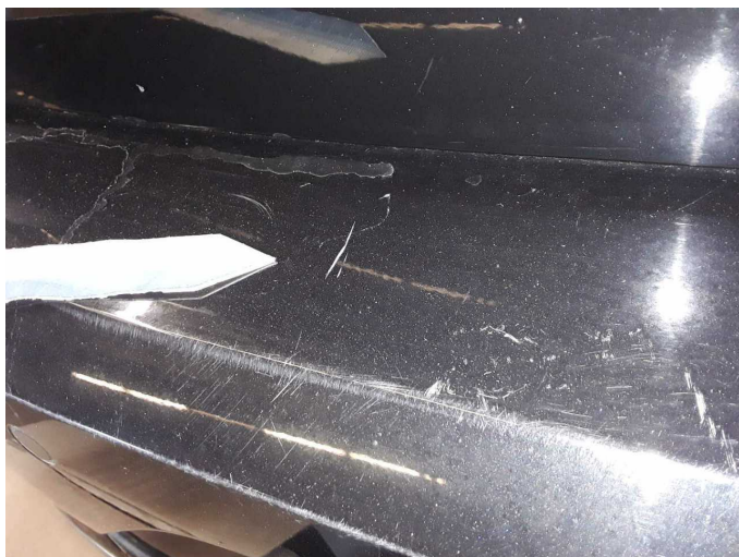
Damage 3: Rear bumper: Rear bumper - Scratch(es) - Paint
