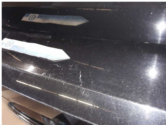
Damage 3: Rear bumper: Rear bumper - Scratch(es) - Paint
