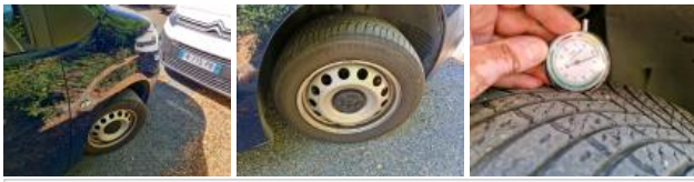
Tyre FL, Out of tolerance, Replace
