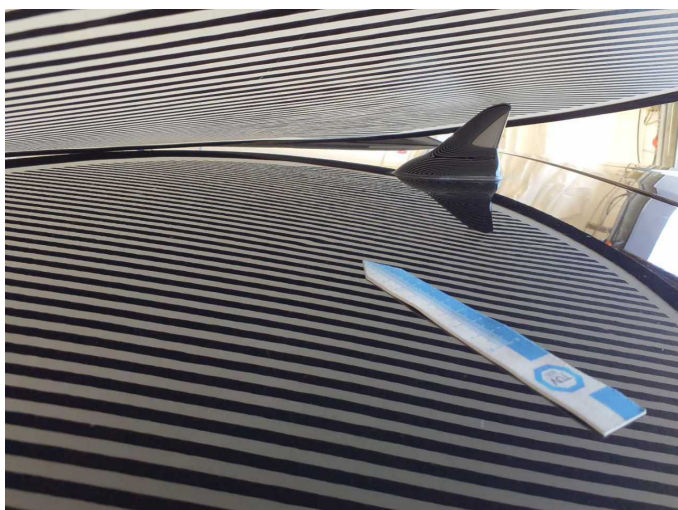
Damage 1: Roof: Roof - dent(s) - Smooth repair work
