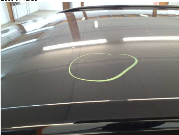
Damage #4: Roof: Roof - dent(s) - Smooth repair work
