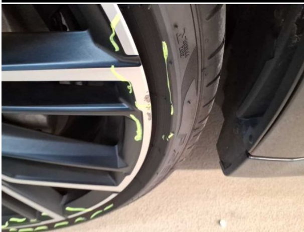
Damage #8: Wheel / tyres: Alloy rim - front left side - Scratched - Loss in value
