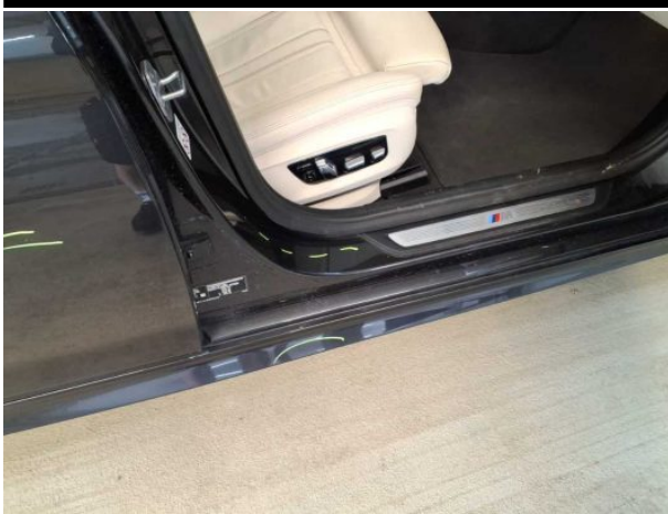
Damage #11: Sill - right side: Sill - Scratched - Smart repair
