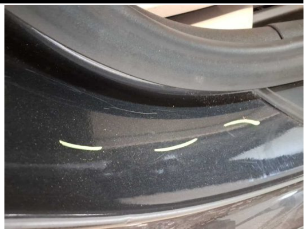
Damage #11: Sill - right side: Sill - Scratched - Smart repair
