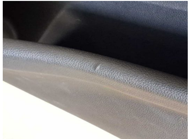
Damage #3: Trim / covers: Door trim - front right side - Damaged - Loss in value
