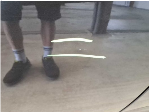
Damage #17: Door - rear right side: Door - Scratched - Repair and paint
