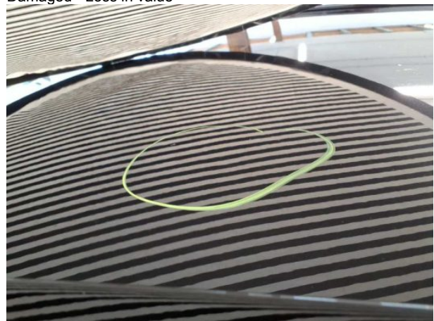
Damage #4: Roof: Roof - dent(s) - Smooth repair work
