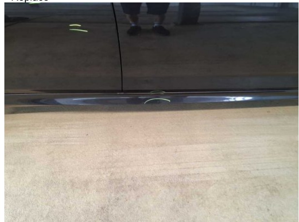
Damage #16: Sill - right side: Trim - Scratched - Repair and paint
