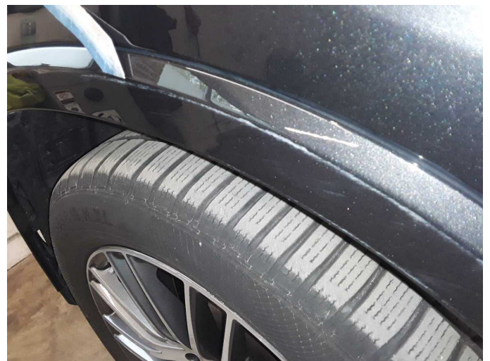
Damage 2: Mudguard - left side: Wheel arch - Scratch(es) - Smart repair
