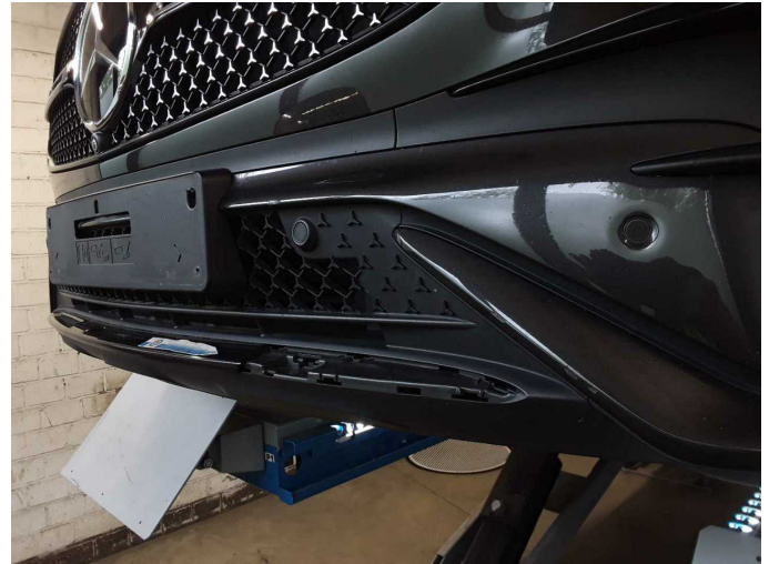
Damage 4: Front bumper: Spoiler - Missing - Replace
