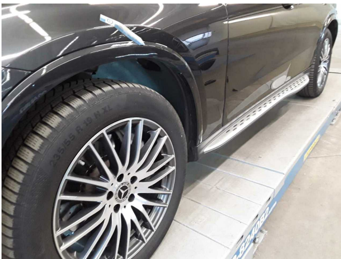
Damage 2: Mudguard - left side: Wheel arch - Scratch(es) - Smart repair
