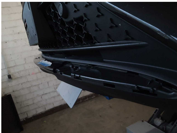
Damage 4: Front bumper: Spoiler - Missing - Replace
