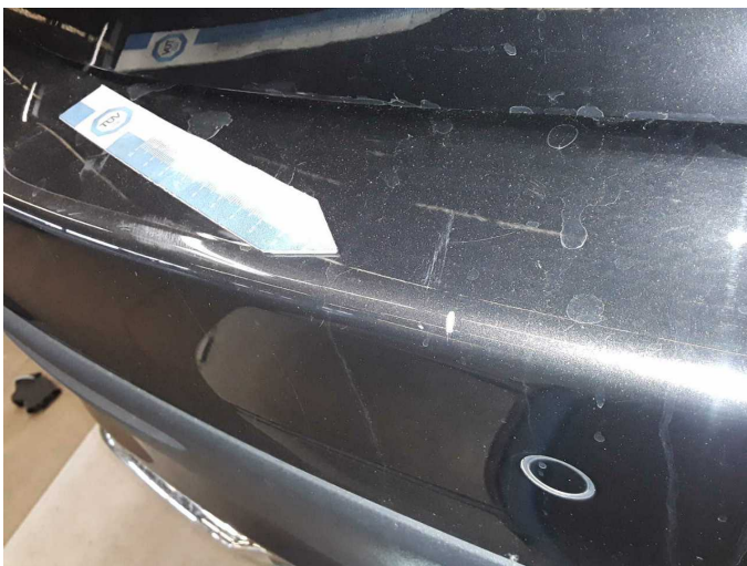
Damage 7: Rear bumper: Rear bumper - Scratch(es) - Paint
