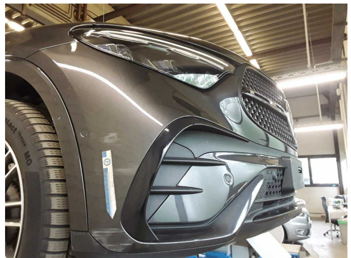
Damage 8: Front bumper: Front bumper - Scratched - Paint
