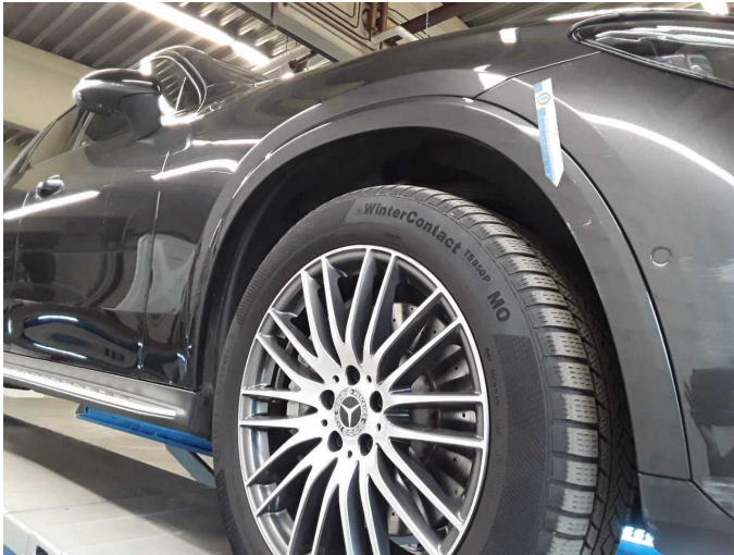
Damage 1: Mudguard - right side: Wheel arch - Scratched - Smart repair
