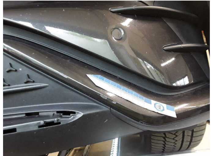
Damage 8: Front bumper: Front bumper - Scratched - Paint
