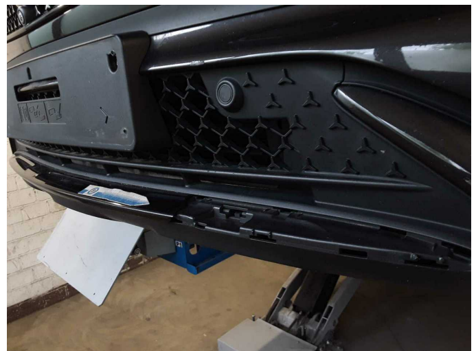
Damage 4: Front bumper: Spoiler - Missing - Replace
