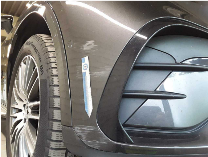
Damage 8: Front bumper: Front bumper - Scratched - Paint
