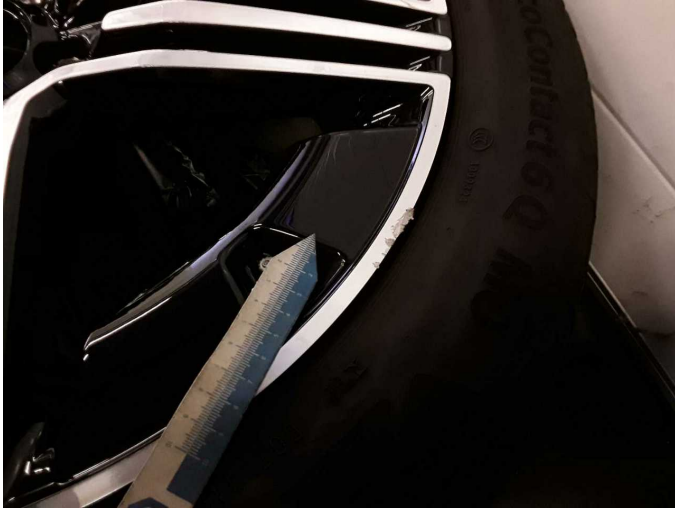
Damage 5: 2nd wheel set: 3 alloy rims - Scratched - Loss in value
