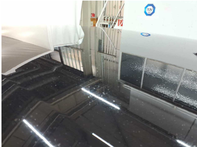
Damage 5: Roof: Roof (Anhaftung hartz) - Paint defect - Paint
