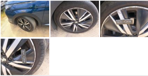
Tyre FL, Out of tolerance, Replace
