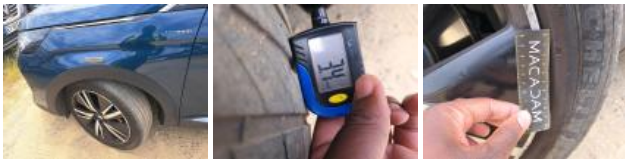
Tyre FR, Out of tolerance, Replace
