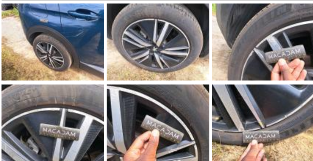
Tyre RR, Tear, Replace
