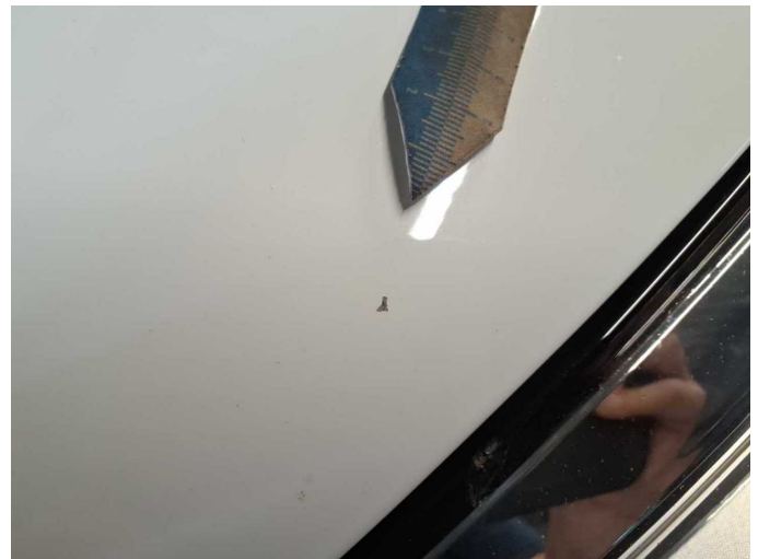
Damage 4: Bonnet: Bonnet - Stone chips - Paint
