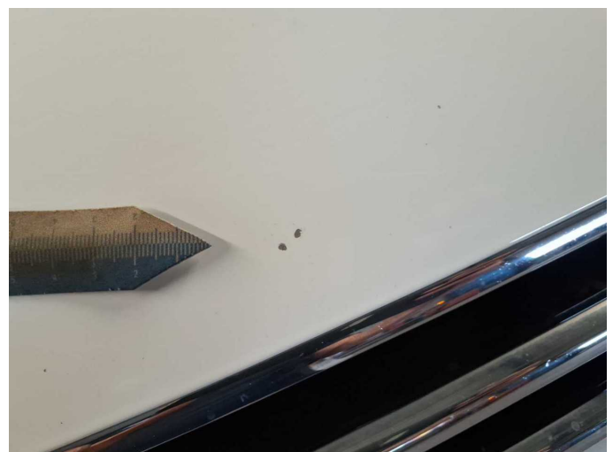
Damage 4: Bonnet: Bonnet - Stone chips - Paint
