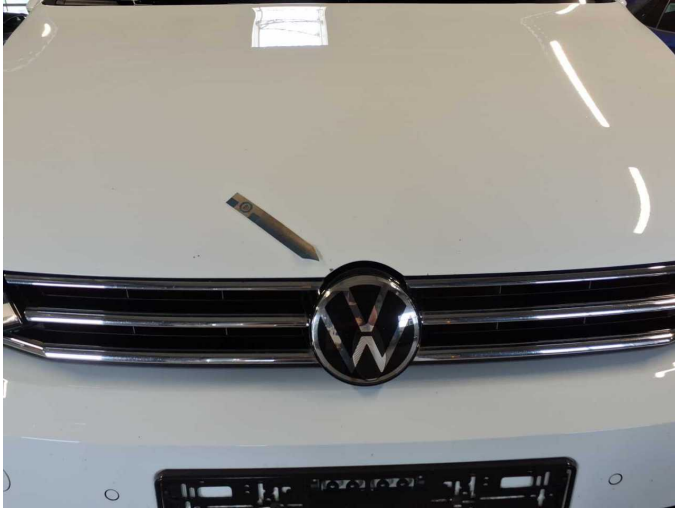
Damage 4: Bonnet: Bonnet - Stone chips - Paint
