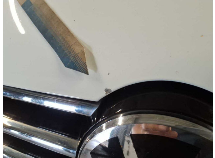
Damage 4: Bonnet: Bonnet - Stone chips - Paint
