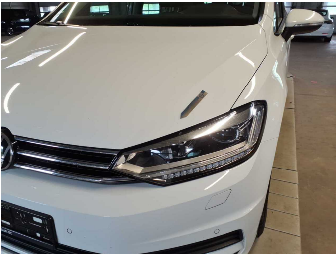
Damage 4: Bonnet: Bonnet - Stone chips - Paint
