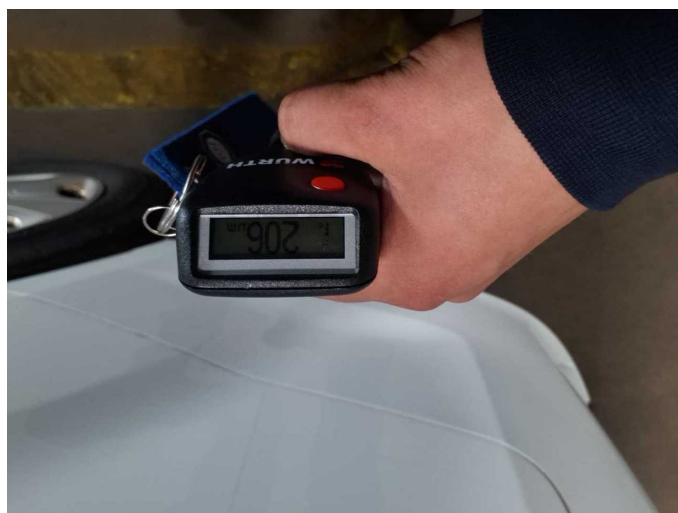
Repainting 1: Side panel - rear right side
