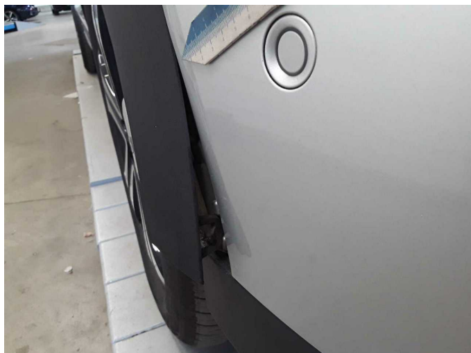
Damage 1: Mudguard - right side: Wheel arch - Loose - Un- / install
