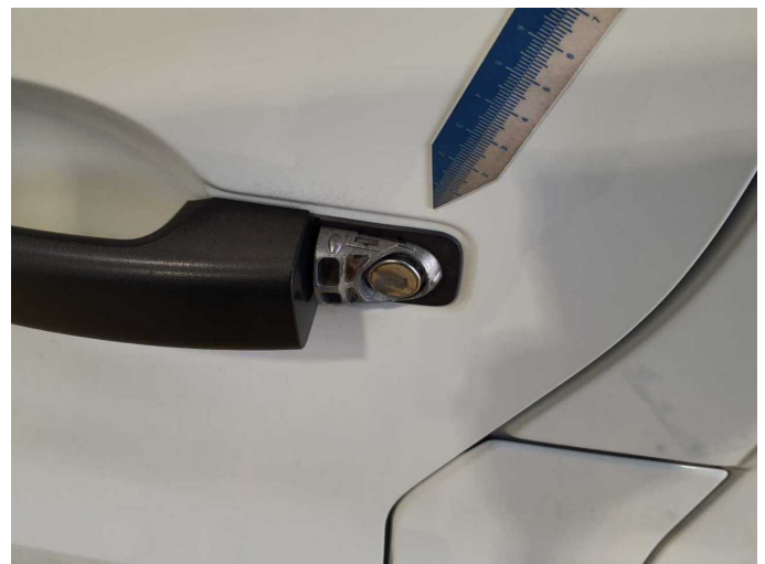
Damage 3: Door - front left side: Door handle - outside - Missing - Replace
