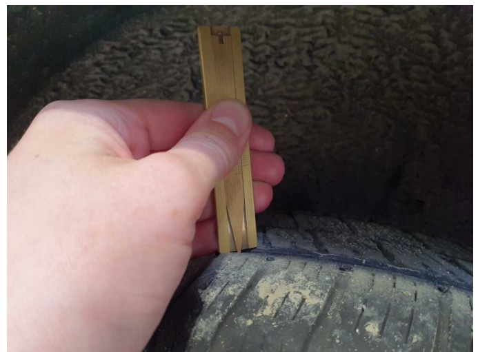
Damage 6: Wheel / tyres: Tyre - right - Worn - Replace
