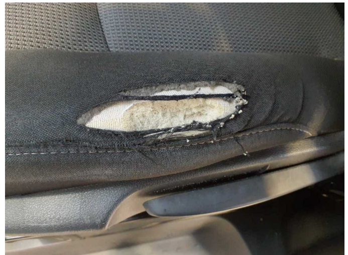
Damage 8: Seat - front: Seat cover - left side (Und polster) - Broken / torn - Replace
