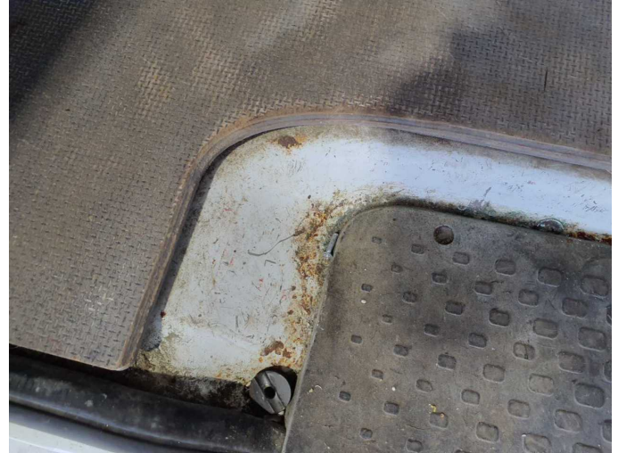
Damage 10: Side panel - rear right side: Sill - Corrosion - Repair and paint
