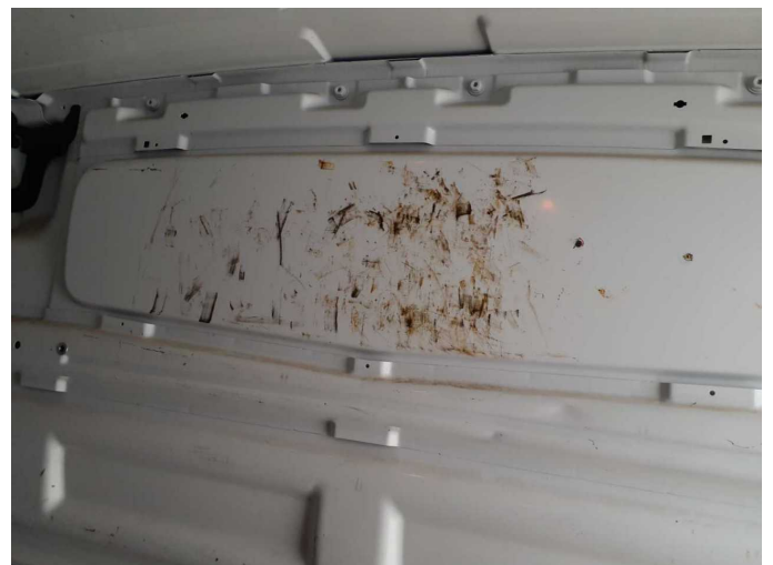
Damage 13: Body: Partition wall - Holes - Replace
