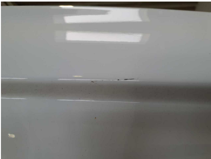
Damage 12: Boot lid / rear door: Rear door - right side - Dent / paintcoat damage - Repair and paint
