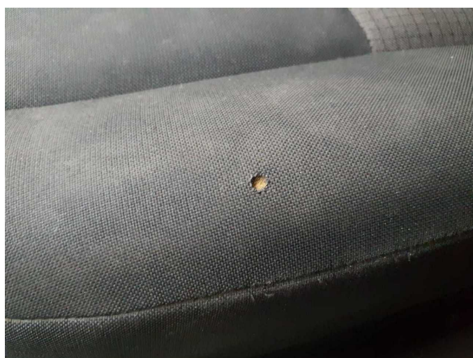
Damage 4: Seat - front: Seat cover - right side - Holes - Smart repair
