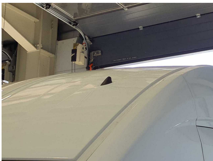
Missing part 1: Roof: Stub aerial - Missing - Replace
