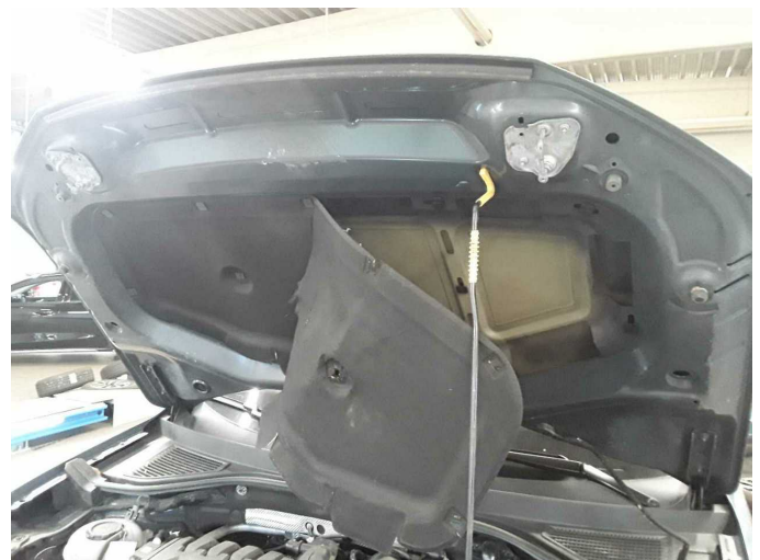
Damage 1: Bonnet: Insulation lining - Damaged - Replace
