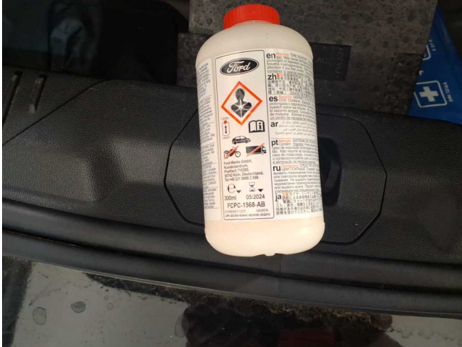
Damage 3: Equipment: Tirefit filler - Expired - Replace
