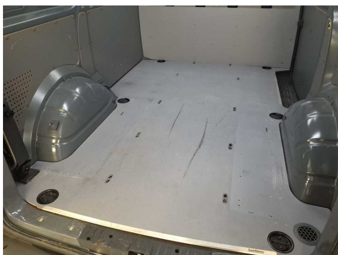
Wear and tear 2: Interior: Cargo area floor - Scratch(es) - No deduction
