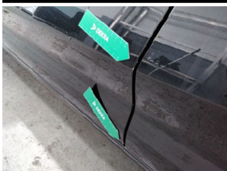
Tür / Vorne Links / Kratzer
