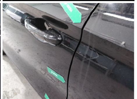
Tür / Vorne Links / Kratzer
