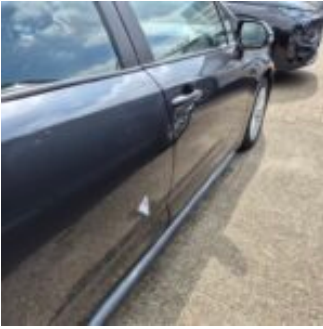
Damage Part Reardoor - Right
