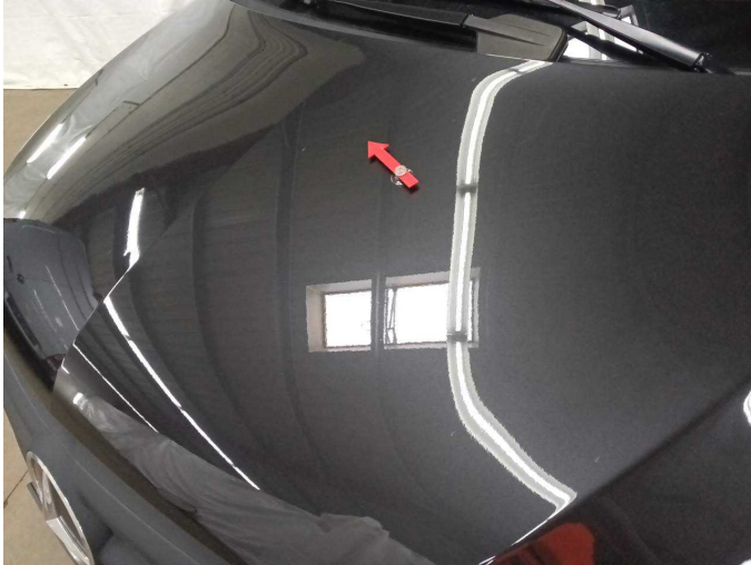
Damage 4: Bonnet: Bonnet - dent(s) - Smooth repair work
