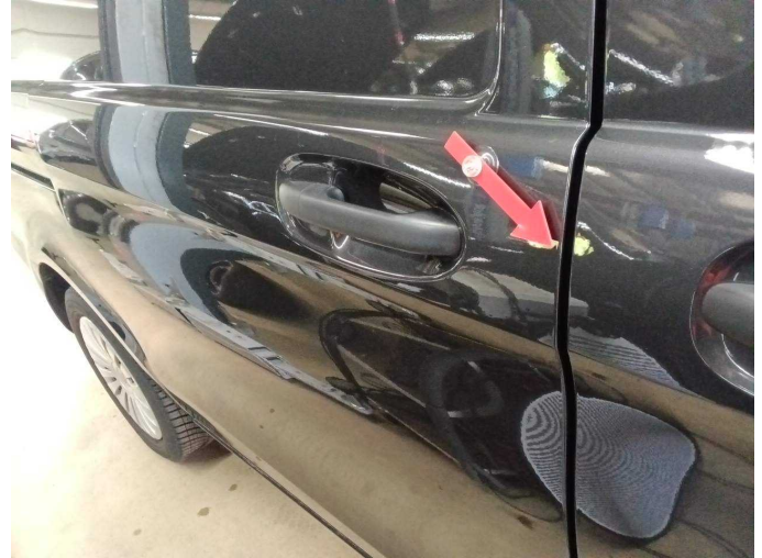
Damage 2: Sliding door, right: Sliding door - Scratch(es) - Smart repair
