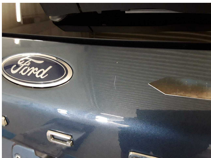
Damage 3: Boot lid / rear door: Boot lid glazed - Dent / paintcoat damage - Smart repair
