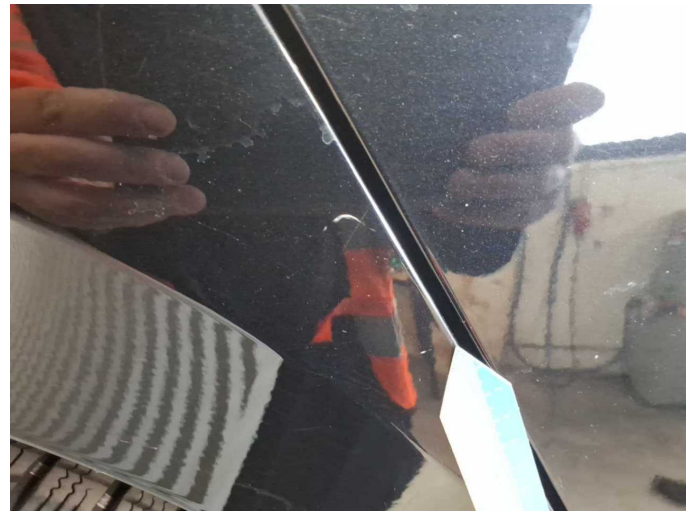
Damage 4: Side panel - rear right side: Side panel - Dent / paintcoat damage - Paint
