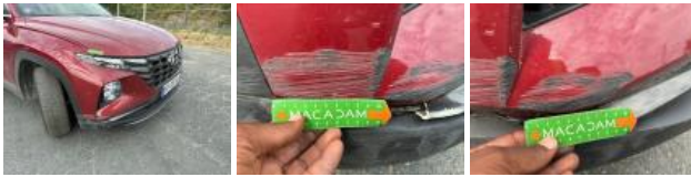
Bumper moulding F, Broken, Replace and paint
