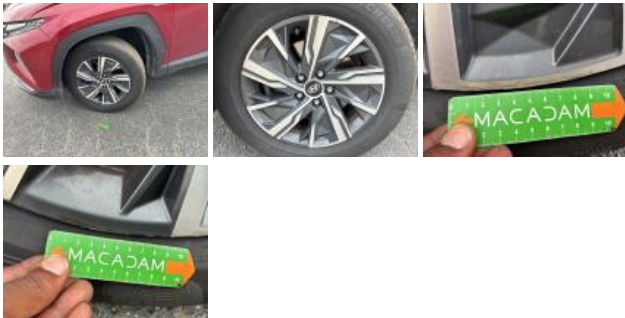
Tyre FL, Out of tolerance, Replace
