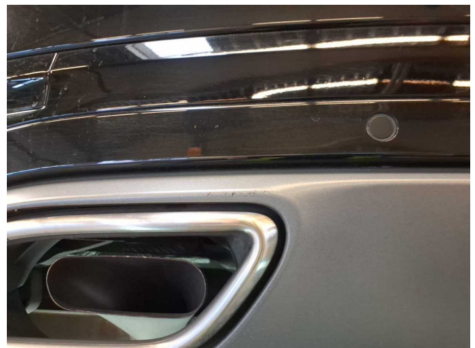
Damage 4: Rear bumper: Spoiler - Scratch(es) - Smart repair
