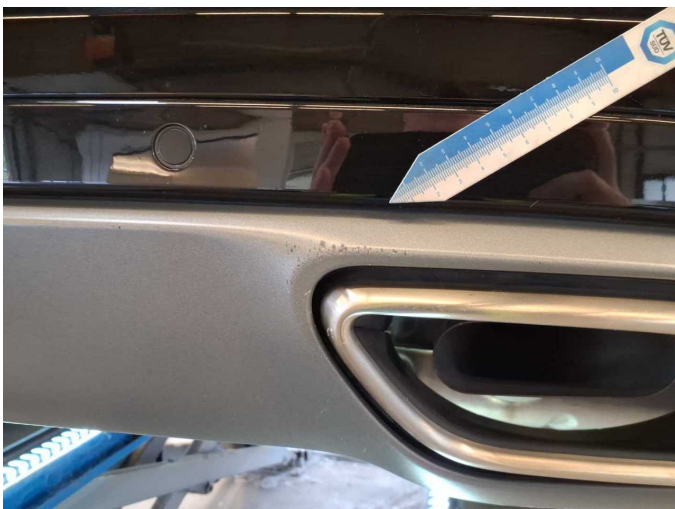
Damage 4: Rear bumper: Spoiler - Scratch(es) - Smart repair
