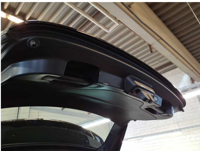
Damage 1: Trim / covers: Boot lid - interior trim - Scratch(es) - Smart repair
