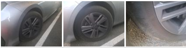
Tyre RL, Out of tolerance, Replace
