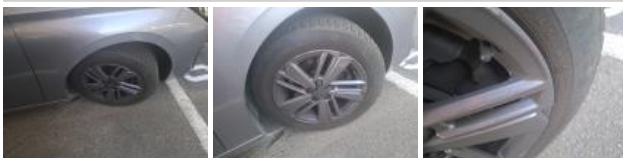
Tyre RR, Out of tolerance, Replace
