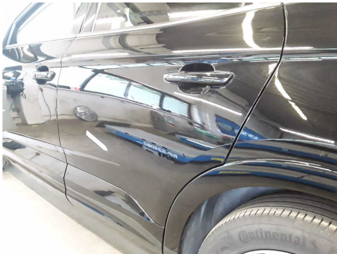
Damage 7: Door - rear left side: Door - Deformed - Repair and paint
