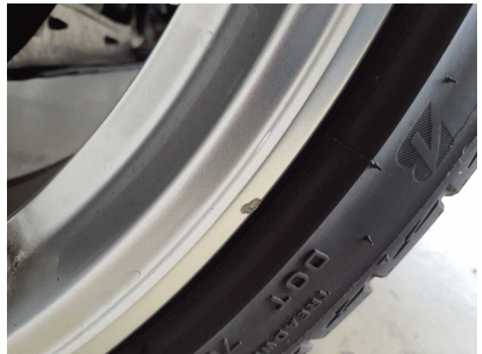
Damage 5: Wheel / tyres: Alloy rim - rear left side - Scratch(es) - Loss in value
