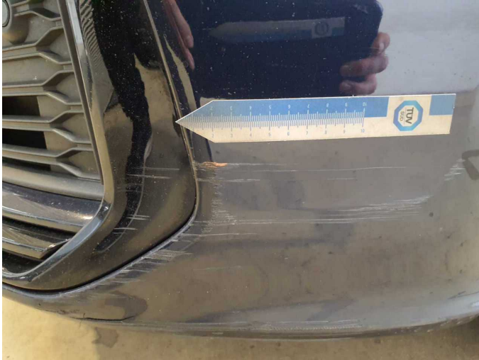
Damage 14: Front bumper: Front bumper (Zusätzlich Blende VL Kratzer) - Scratch(es) - repair according to calculation
