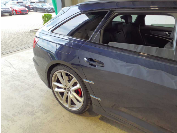
Damage 12: Side panel - rear right side: Side panel - Deformed - Repair and paint
