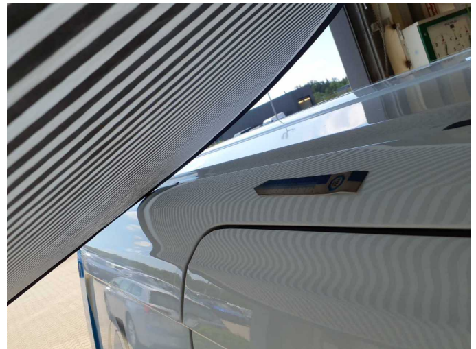
Wear and tear 12: Roof: Roof rail - right side - dent(s) - Smooth repair work
