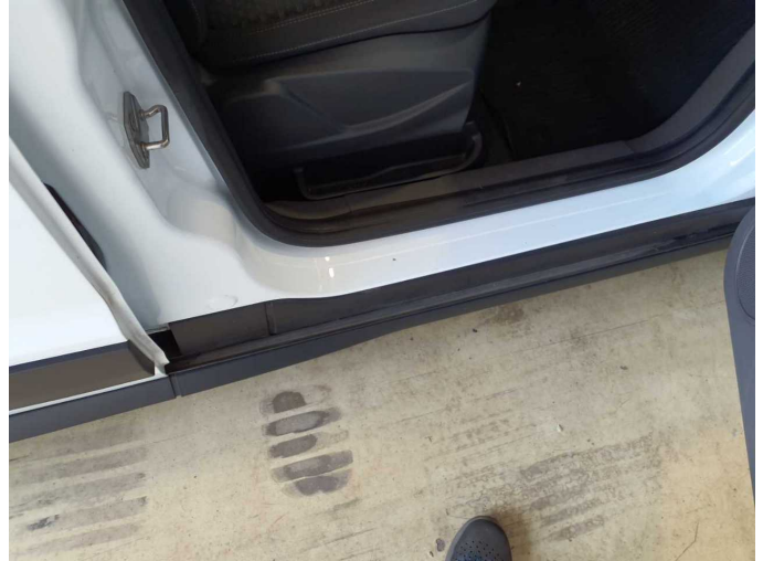
Wear and tear 8: Sill - right side: Sill - Scratch(es) - Cover / polish
