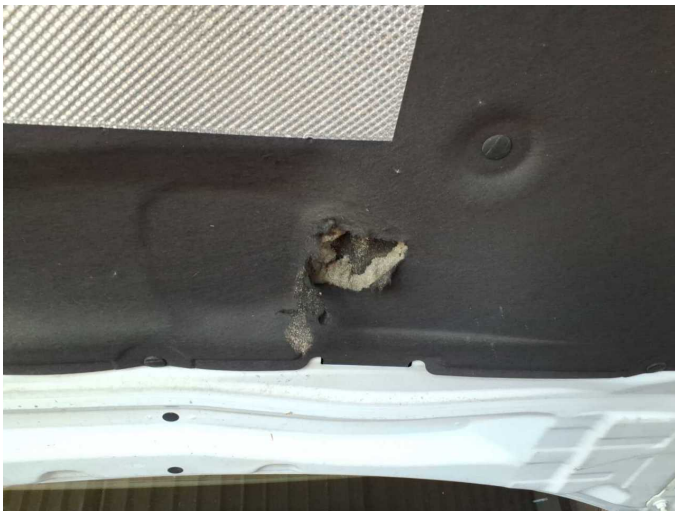
Damage 10: Bonnet: Insulation lining - Damage caused by marten / rodent - Replace
