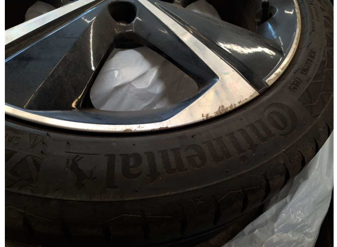
Damage 20: 2nd wheel set: Alloy rim set - complete - Scratch(es) - Replace
