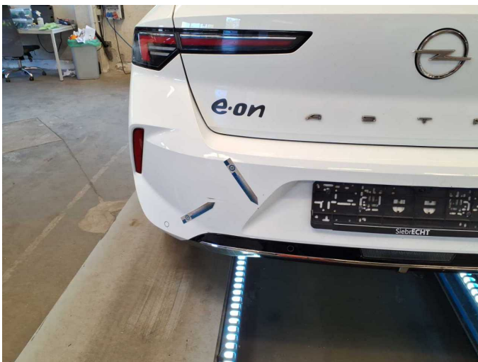
Damage 17: Rear bumper: Rear bumper - Scratch(es) - Paint
