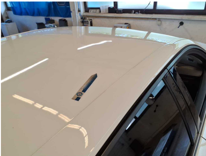
Damage 19: Roof: Roof - Dent / paintcoat damage - Repair and paint
