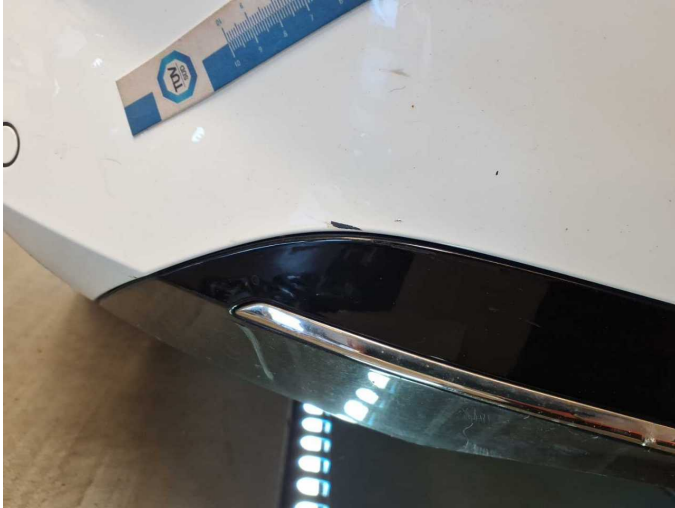
Damage 17: Rear bumper: Rear bumper - Scratch(es) - Paint
