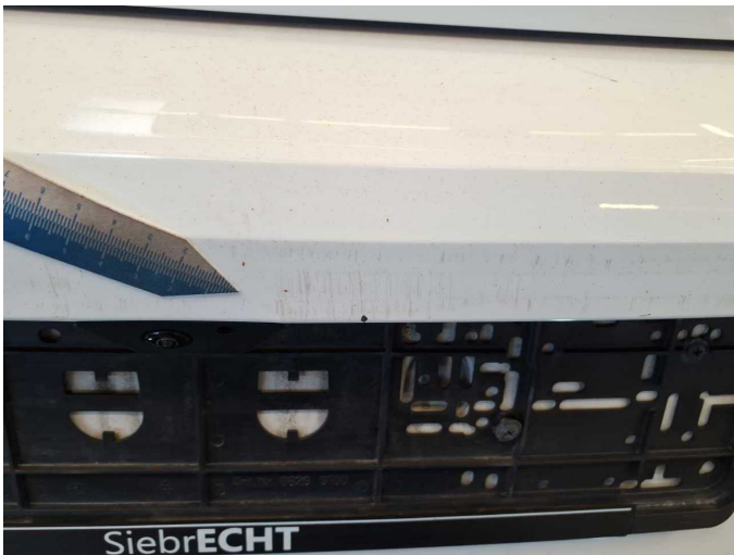
Damage 17: Rear bumper: Rear bumper - Scratch(es) - Paint
