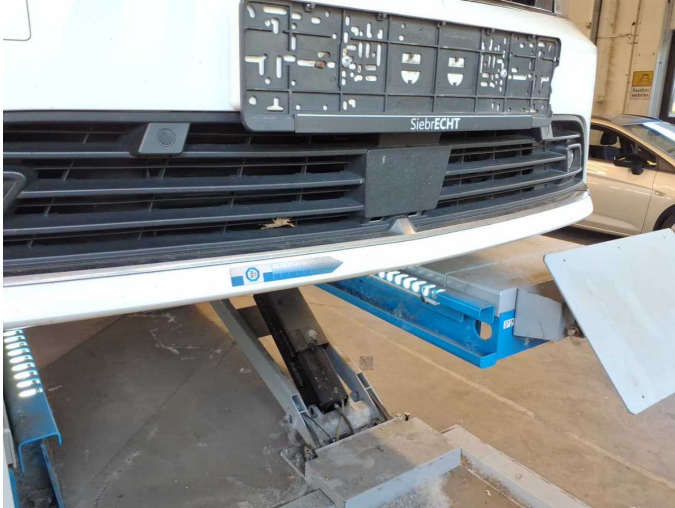
Damage 18: Front bumper: Front bumper - Scratch(es) - Paint
