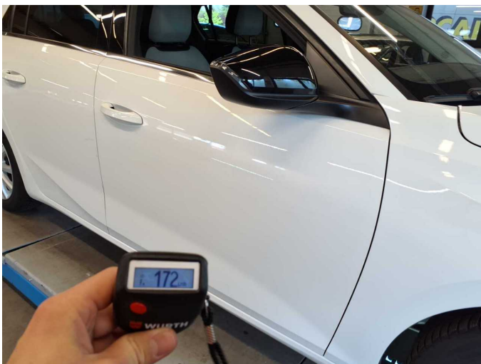
Repainting 4: Door - front right side
