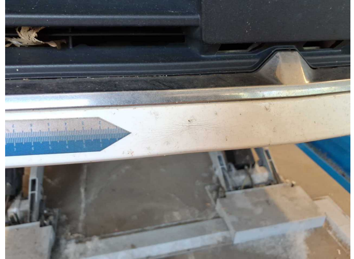
Damage 18: Front bumper: Front bumper - Scratch(es) - Paint
