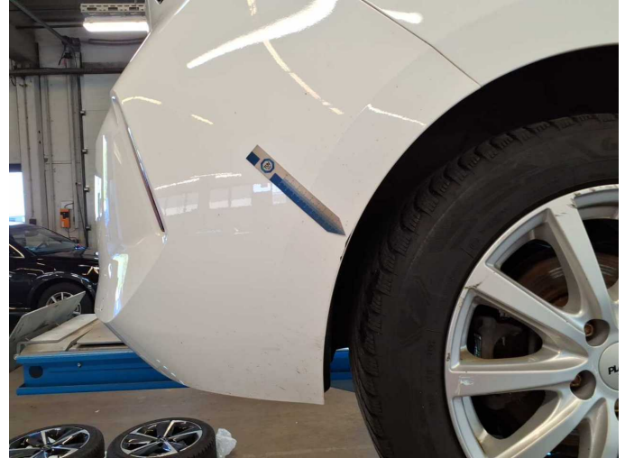
Damage 17: Rear bumper: Rear bumper - Scratch(es) - Paint
