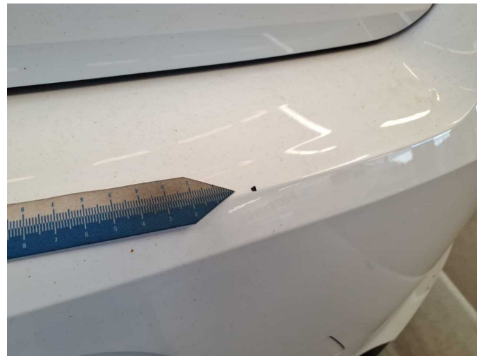
Damage 17: Rear bumper: Rear bumper - Scratch(es) - Paint
