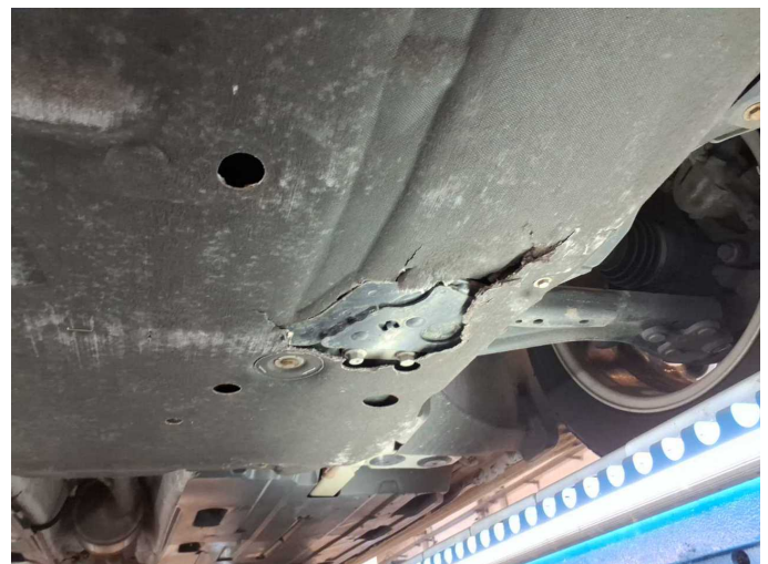
Damage 14: Engine: Engine cowling - lower - Broken / torn - Replace
