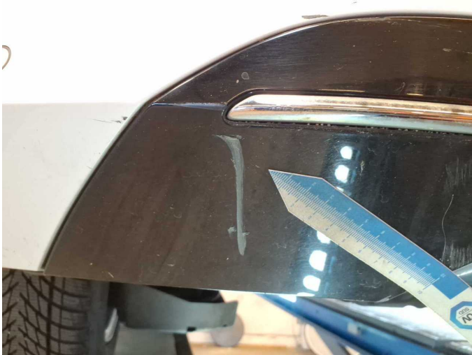
Damage 16: Rear bumper: Spoiler - Scratch(es) - Paint
