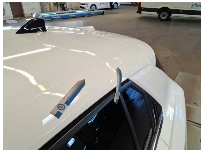
Damage 9: Roof: Roof rail - left side - dent(s) - Smooth repair work
