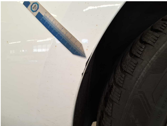
Damage 17: Rear bumper: Rear bumper - Scratch(es) - Paint
