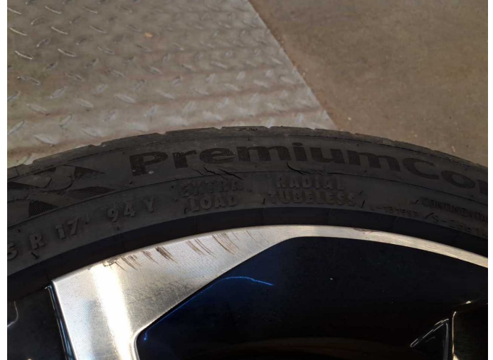
Damage 6: 2nd wheel set: 1 tyre - Damaged - Replace
