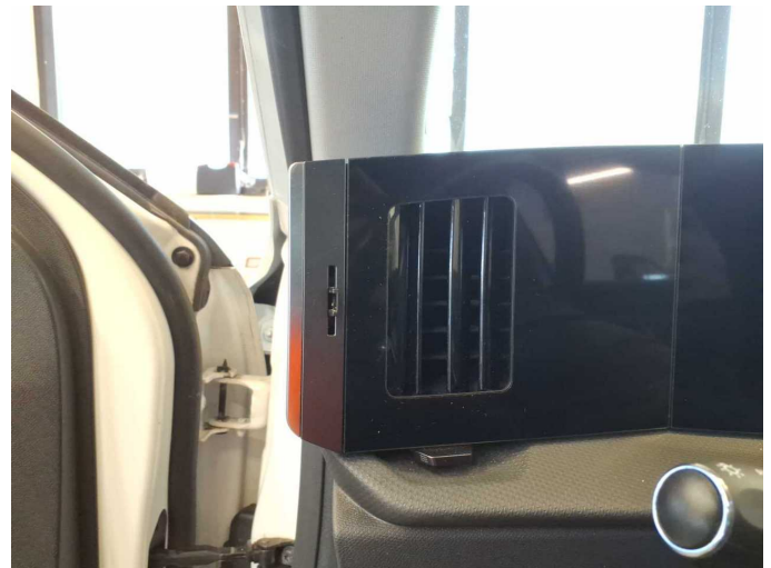
Damage 8: Trim / covers: Trim / covers (Lüftungsgitter verstellhebel) - Missing - Replace
