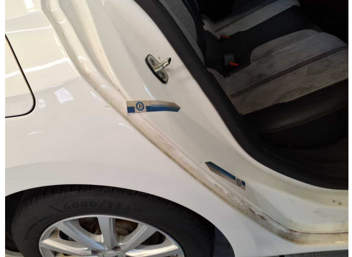
Damage 13: Side panel - rear right side: Sill - Dent / paintcoat damage - Smart repair
