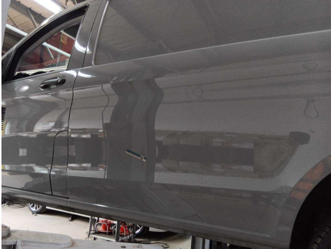
Damage 3: Side panel - rear left side: Side panel (1) - dent(s) - Smooth repair work
