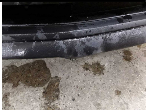
Damage #6: Front bumper: Spoiler - Deformed - Replace
