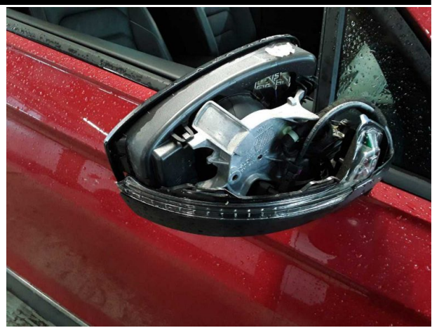
Damage #4: Wing mirror - right side: Mirror housing - Loose - Diagnosed and repair if necessary
