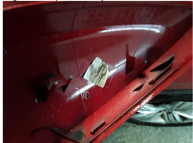
Damage #5: Wing mirror - right side: Cap - Loose - Replace
