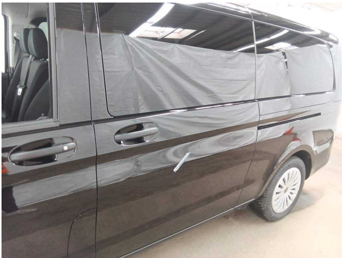
Damage 5: Sliding door - left side: Sliding door - Dent / paintcoat damage - Repair and paint
