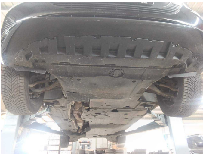
Wear and tear 2: Body: Underbody panelling - Scratch(es) - No deduction
