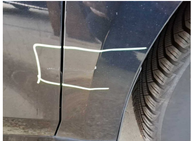
Damage #6: Mudguard - right side: Mudguard - right side - Scratched - Repair and paint
