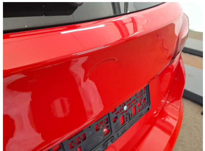
Damage 2: Boot lid / rear door: Emblem - Missing - Replace
