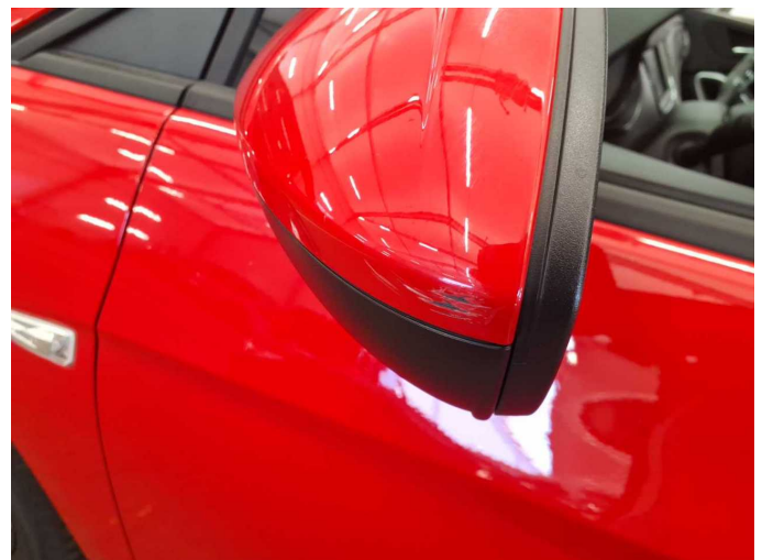
Damage 5: Wing mirror - left side: Cap - Scratch(es) - Paint
