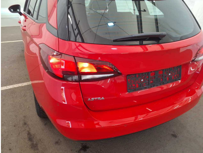
Damage 6: Tail light: Tail lamp - left side - Leaking - Replace
