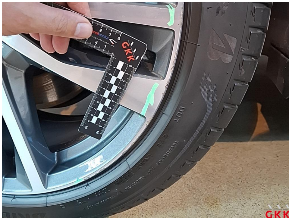
Picture 23 LM wheel, rear right, scratched, replace
