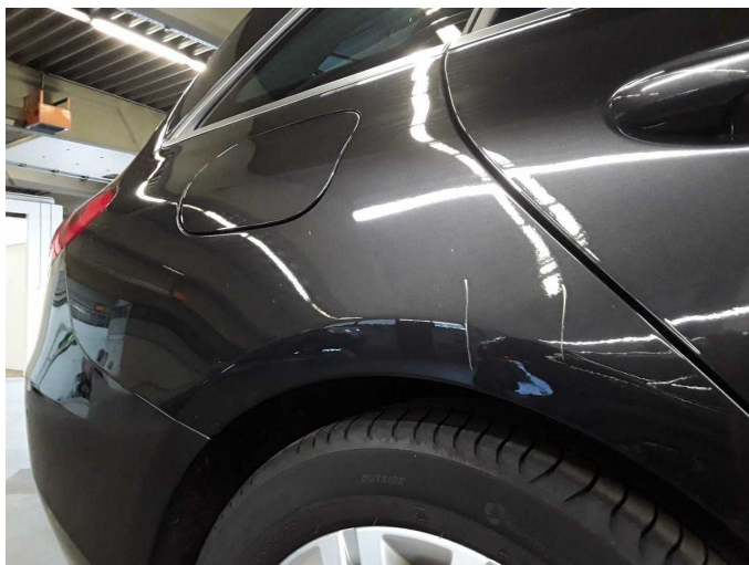
Wear and tear 4: Side panel - rear right side: Side panel - dent(s) - No deduction
