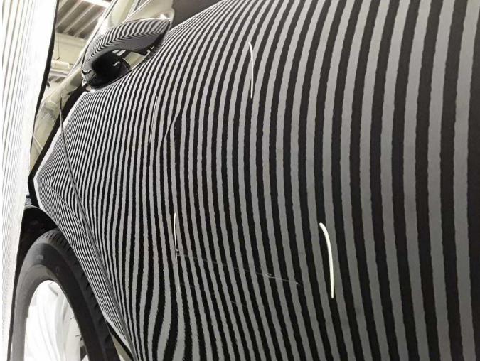
Damage 2: Door - rear right side: Door - Dent / paintcoat damage - Repair and paint
