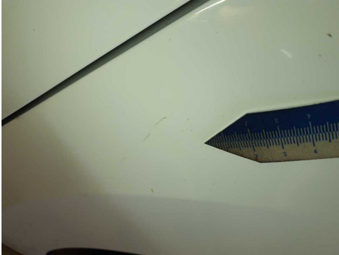
Damage 10: Side panel - rear left side: Side panel - Dent / paintcoat damage - Smooth repair work
