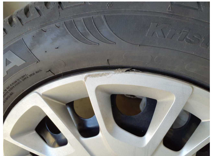
Damage 3: 2nd wheel set: 1 wheel cover - Broken / torn - Replace
