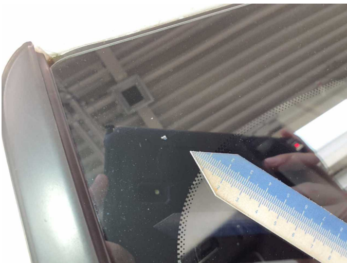
Damage 14: Vehicle glazing: Windscreen - Stone chips - Replace
