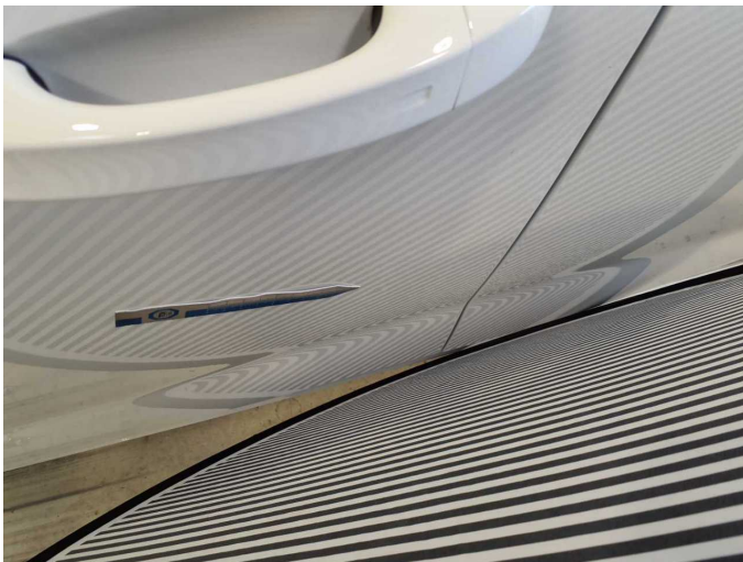
Damage 6: Door - front left side: Door - Dent / paintcoat damage - Smart repair
