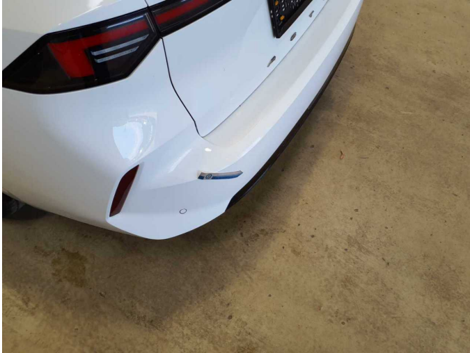
Damage 15: Rear bumper: Rear bumper (gestaucht) - Dent / paintcoat damage - Repair and paint
