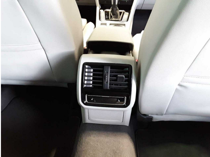
Damage 2: Instrument panel: Air nozzle - centre (Versteller fehlt) - Differs from the original configuration - Replace
