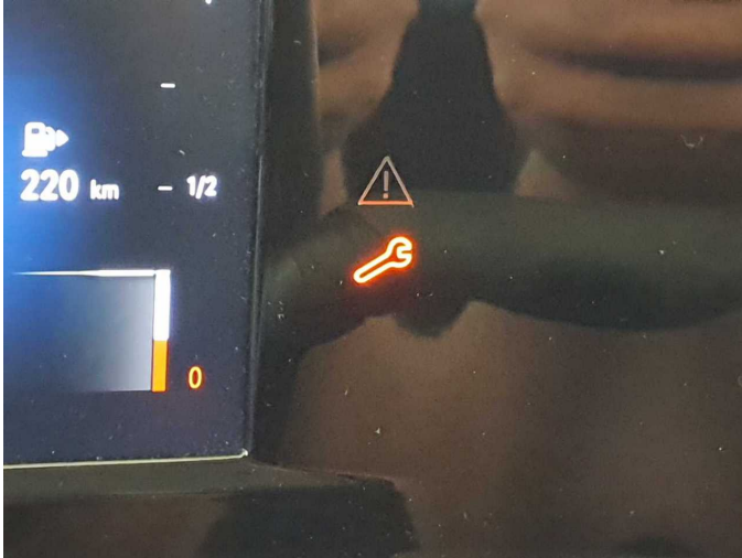
Damage 3: Misc.: Inspection / maintenance - Due - Perform
