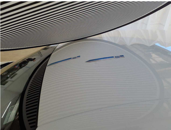
Damage 2: Roof: Roof (6 Dellen) - dent(s) - Smooth repair work
