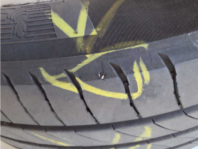
Damage 1: 2nd wheel set: 1 tyre - Damaged - Replace
